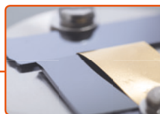
Two XPS samples on a sample holder - one masked with Au foil.
