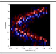
**Figure 3:** The high efficiency of the system makes it possible to make a spin resolved overview measurement of in this case the complete ThetaY cut in only 1 hour.
