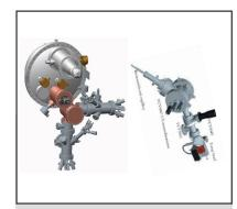
Key equipment: DA30-L equipped with a 2D/3D Ferrum VLEED detector system and the VUV5k UV source.
