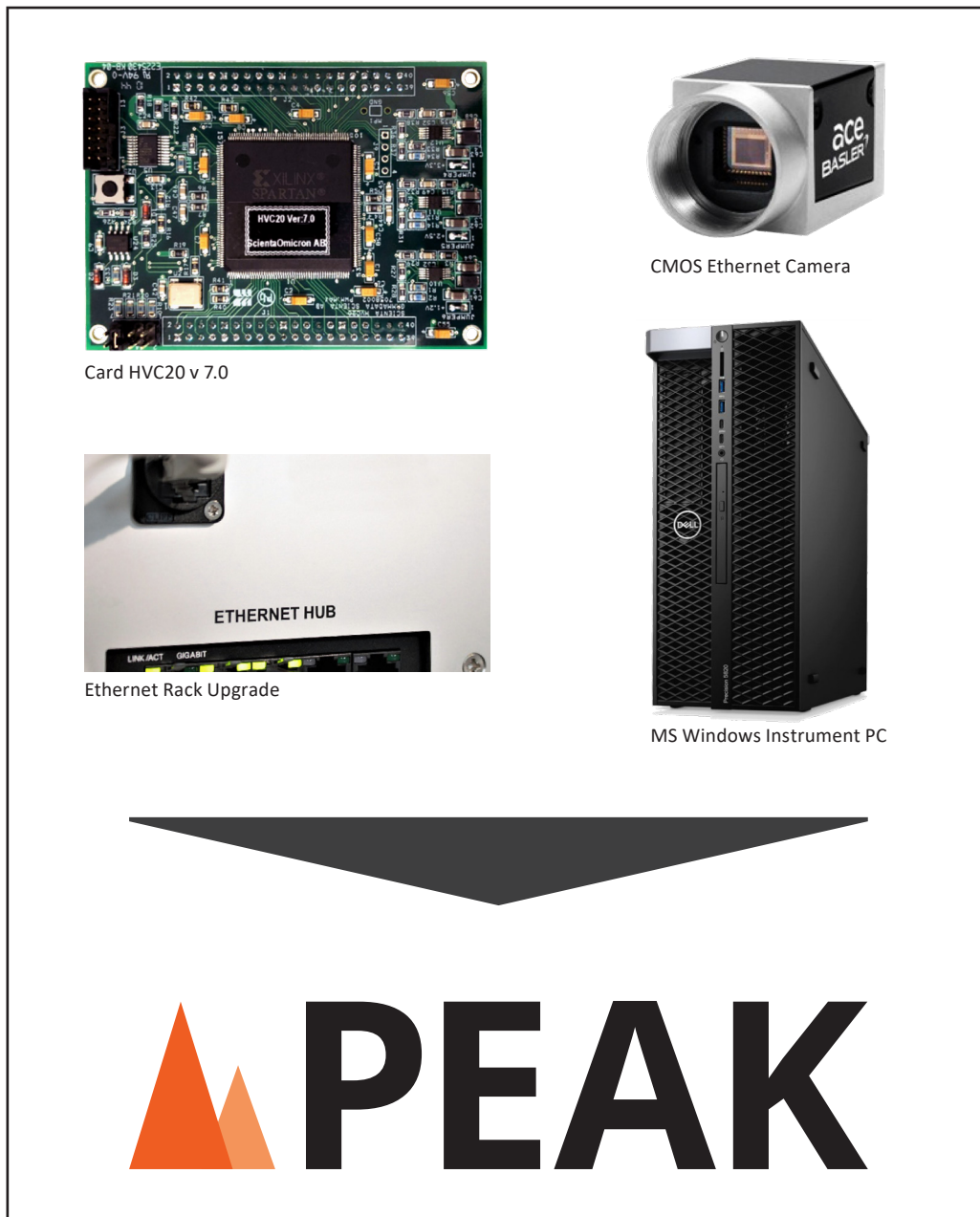
Figure 7: The analyser control upgrade package brings the HV rack communication, detector camera, and the instrument PC to the latest standard. With this the PEAK minimum requirements are satisfied and extend the life of older generation analysers.
